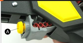
In order to guarantee accurate crimping, turn the knob (A) clockwise for small size ferrules (0.50 mm<sup>2</sup> to 0.75 mm<sup>2</sup>) or counterclockwise for larger sizes (1.00 mm<sup>2</sup> to 2.50 mm<sup>2</sup>).
