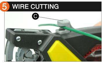
• Place wire inside the cutting jaws (C) and close tool's handles.
