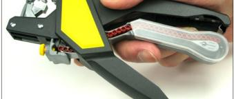
• Cartridge can be easily removed by pulling it away from the handle. To insert the cartridge, place its tip toward the inside of the tool and push cartridge upwards toward handle. All cartridges can house any size ferrule.
