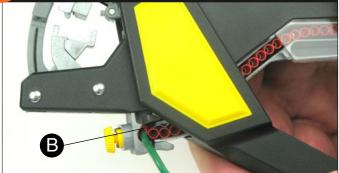
• Insert wire inside the ferrule (B), making sure wire strands are securely housed inside the ferrule's pin. Close tool's handles with moderate force in order to detach the ferrule from the strip.
